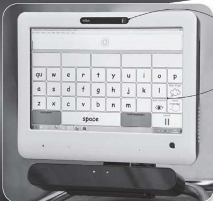
internal web cam allowing head tracking
