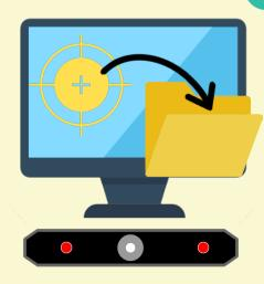
Calibrate the learner's eyes within the eye tracker setup software and save their User Profile. You do not have to re-calibrate every time they use the eye tracker. Just check their User Profile is selected. Individual points can be improved if required.
